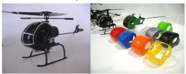
This simple scale kit contains the scale body, fins and a set of trim and logo decals. The cost of the kit (including delivery) is likely to be around £16\*. This body kit will work with the stock Blade mSR skids but works and looks best with the TUFF LG Kit available separately (as shown above). The TUFF LG kit contains a fibreglass parts tree, 2 TUFF struts, 2 skids, 2 rubber spacers, 2 Nylon screws & 2 rubber battery straps and will be around £16\*
